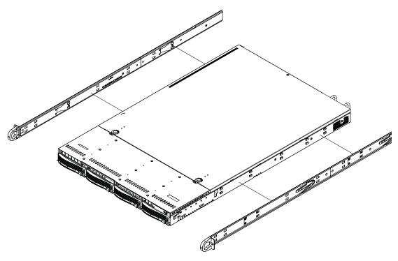
Figure 2-2. Installing the Rack Rails
